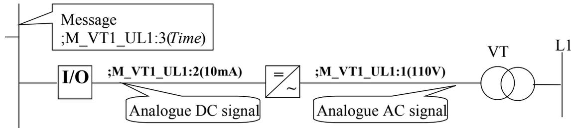
**Figure 7** Part of an analogue signal
