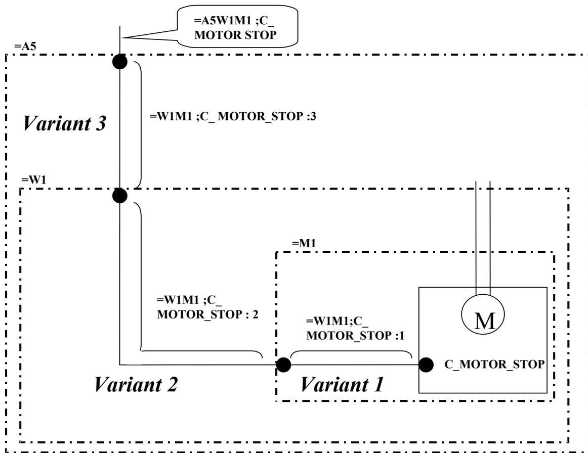
Figure 16 Signal variants in a Signal connection
