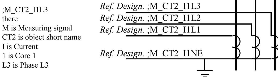
**Figure 4 Example of Measuring signal**
