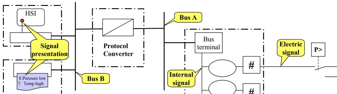
**Figure 14 Typical signal flow (or signal connection chain)**
