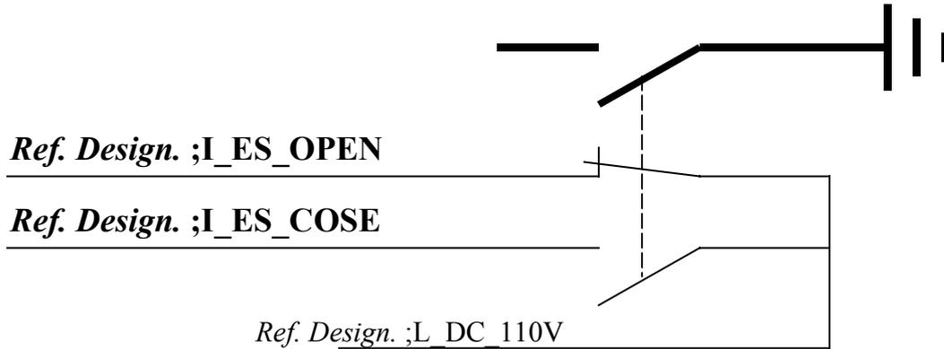
**Figure 2 Example of an Indication signal**
