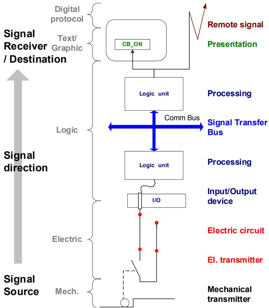
Figure 1 Typical signal connection in a plant, Reporting signal
