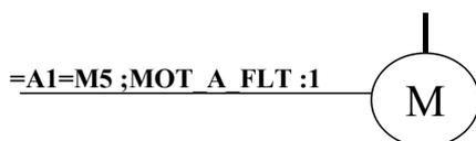
**Figure 24** Example of signal designation corresponding to conformance class 3
