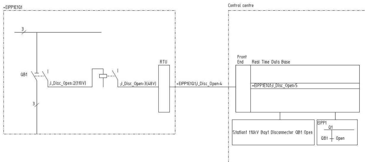
**Figure 21** Indication of status for a disconnector, reporting signal class ( I )
