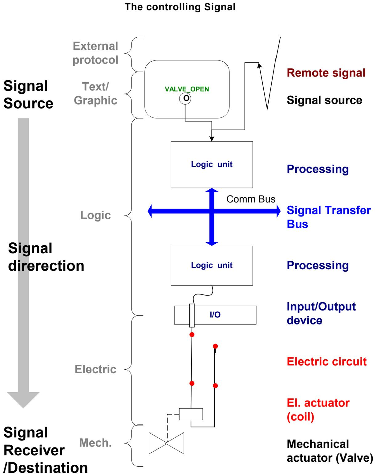
Figure 9 Typical signal chain in a plant, Controlling signal
