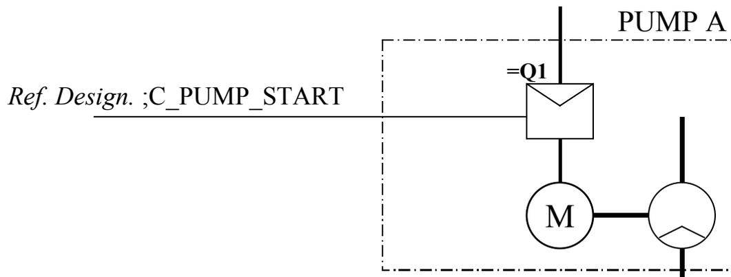
Figure 10 Example of Command signal
