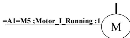
**Figure 23** Example of signal designation corresponding to conformance class 2
