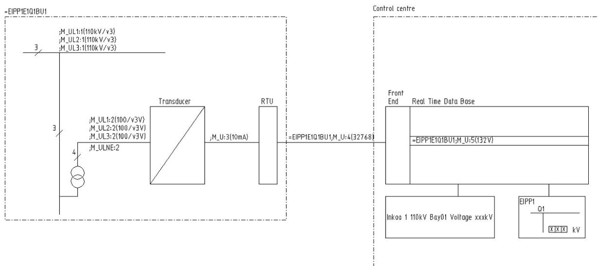
**Figure 20 Voltage measurement, reporting signal class ( M )**
