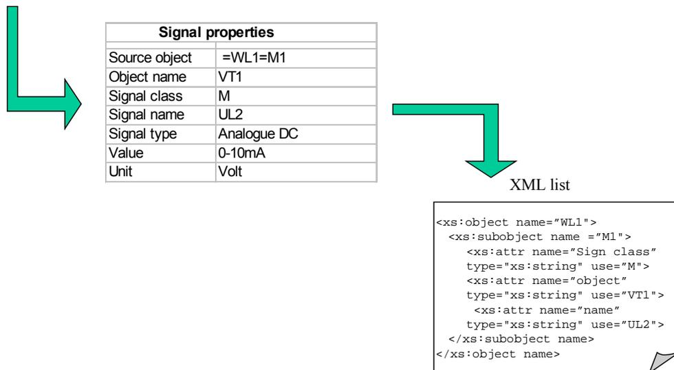
Figure 19 Signal designation presented in Signal properties and XML list
